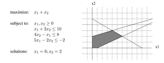
Figure 5.1: A linear program with two variables
